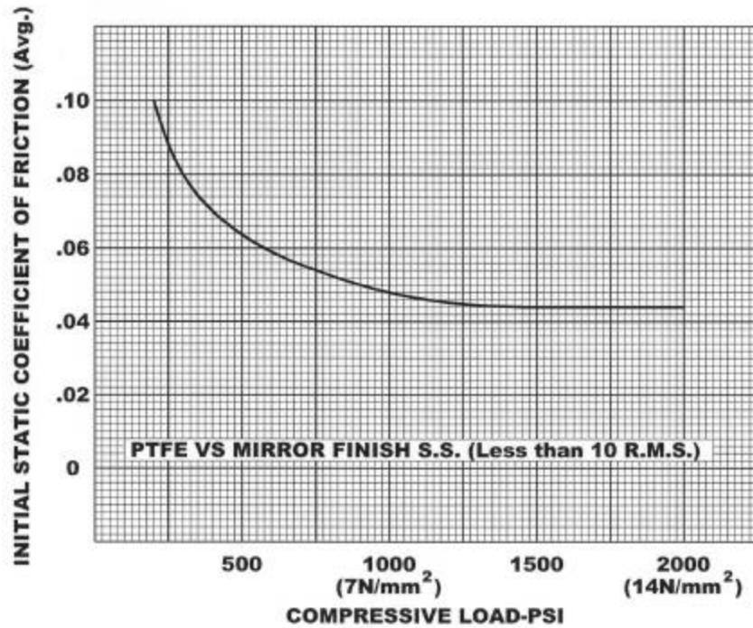
Note: Friction reduces as the compressive stress is increased.
