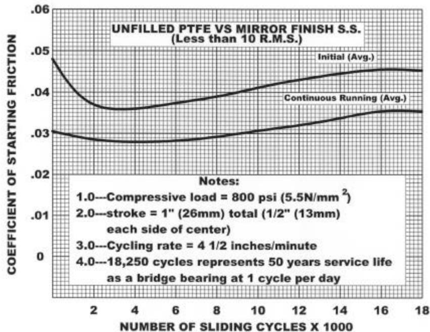
Note: Initial starting friction reduces to a run-in value under continuous sliding conditions.
